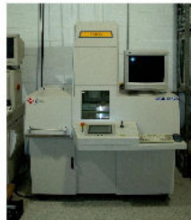
A look at Pro-Tech's X-Ray machine for BGA inspection
